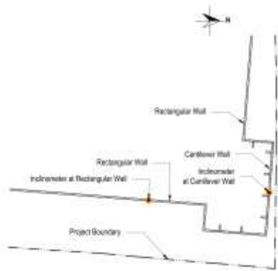
Fig. 7. Location of inclinometers at T shaped cantilever and rectangular wall
