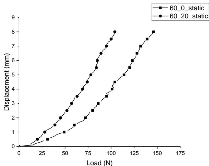
**Fig. 8.** Load-Deflection curve for 60% relative density for horizontal and sloping ground.
