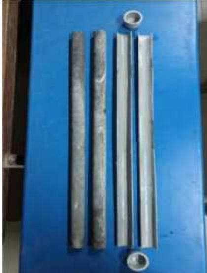
**Fig. 1.** Concrete model piles with mould.
