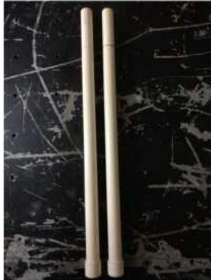
**Fig. 2.** CPVC model piles used in testing.
