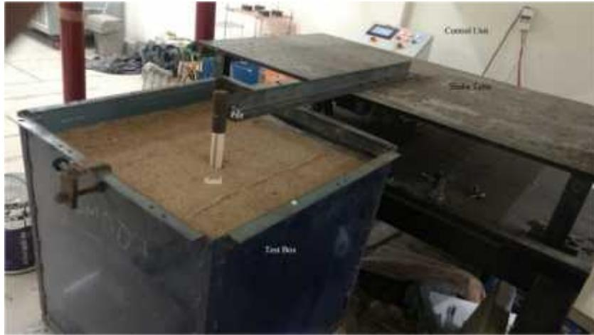
**Fig. 4.** Cyclic loading test arrangement with connections.
