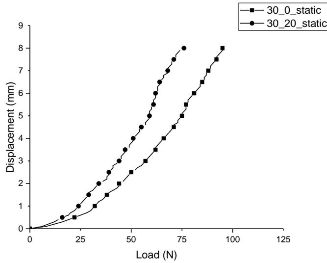
**Fig. 7.** Load-Deflection curve for 30% relative density for horizontal and sloping ground.
