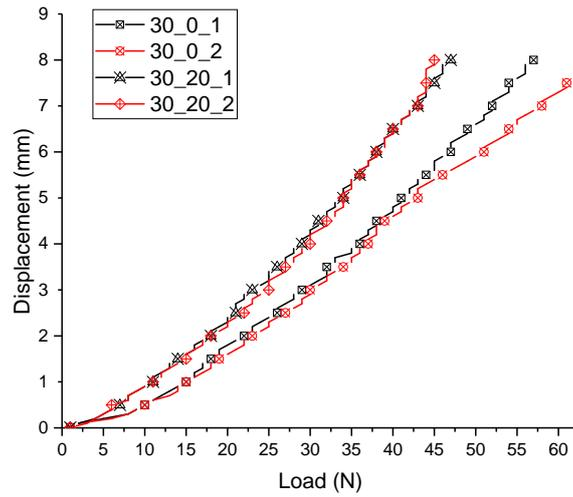
**Fig. 9.** Load-deflection curve for 30% relative density for cyclic tests.
