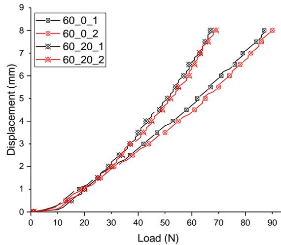
**Fig. 10.** Load-deflection curve for 60% relative density for cyclic tests.
