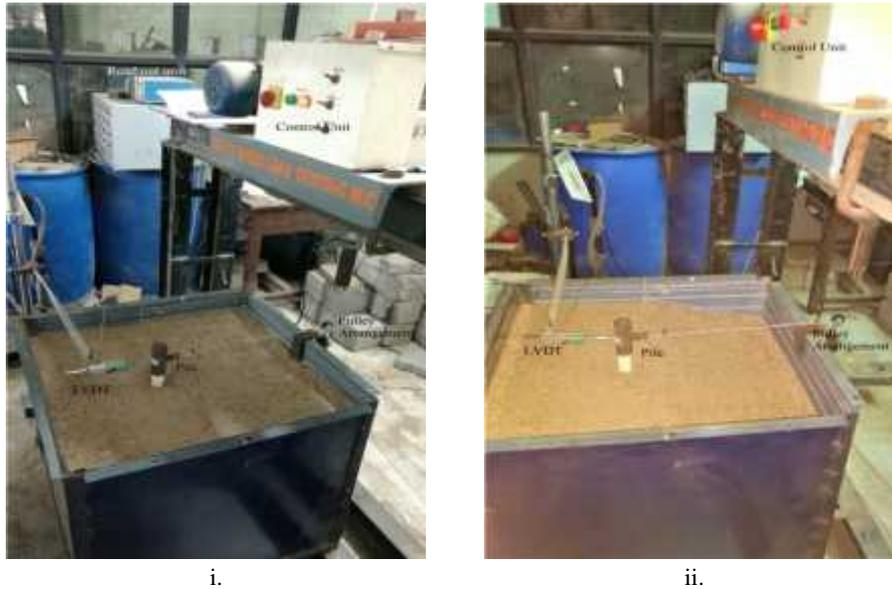
**Fig. 3.** Static loading test set up for i) horizontal ground and, ii) sloping ground.
