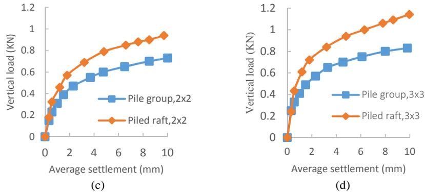
**Fig. 5.** Vertical load-displacement curve of (a) Single pile and pile groups (b) Unpiled raft and piled rafts (c) Pile group and piled raft of 2×2 configuration (d) Pile group and piled raft of configuration 3×3
