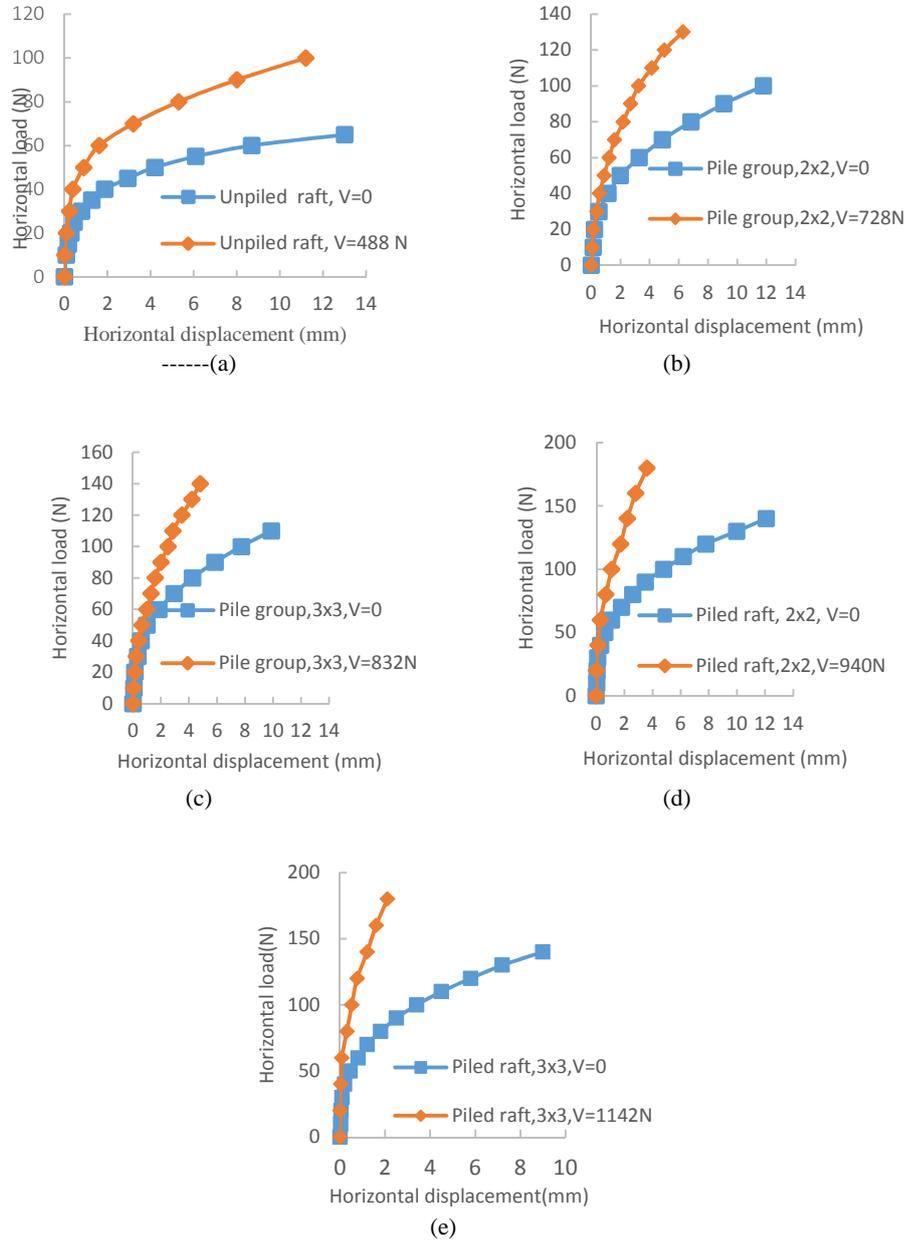
**Fig. 6.** Horizontal load-displacement behavior of a) Un-piled raft b) Pile group of 2x2 configuration c) Pile group of 3x3 configuration d) Piled raft of 2x2 configuration e) Piled raft of 3x3 configuration in presence of vertical load
