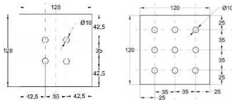
Fig. 2. Piled raft models layout of 2x2 and 3x3 configurations (All the dimensions are in mm)
