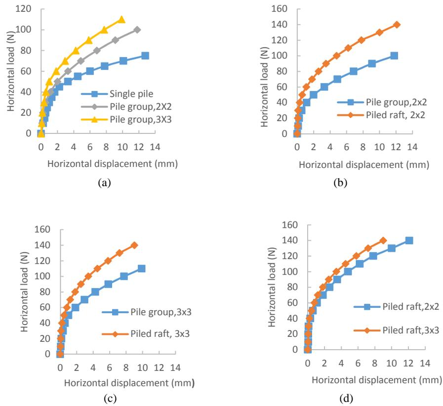
**Fig. 4.** Horizontal load-displacement graphs: a) Single pile and pile groups b) Pile group and piled raft of configuration 2×2 c) Pile group and piled raft of configuration 3×3 d) Piled rafts of configuration 2×2 & 3×3
