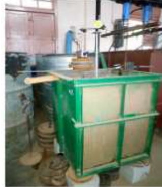
Fig. 2. View of model tank with provision apply vertical and lateral load
