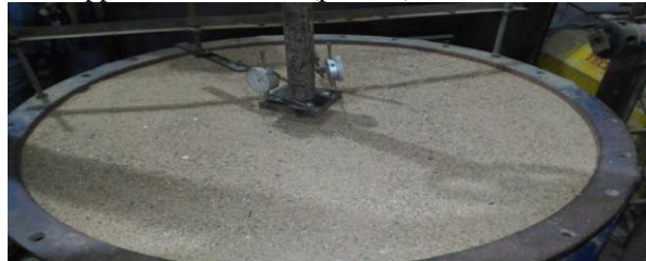
Fig.1. Final setup of pile load testing program.
