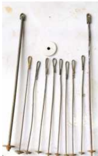
Fig. 5 Anchor Piles used in laboratory Tests
