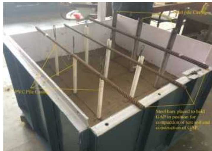
Fig.6. Preparation of test bed and construction of GAP
