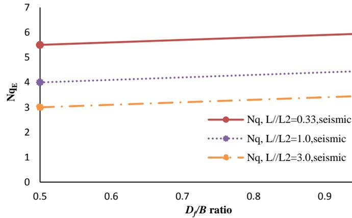
**Fig. 10.** variation of  $N_{qE}$  with  $D_f/B$  ratio with varying layer thickness at seismic condition
