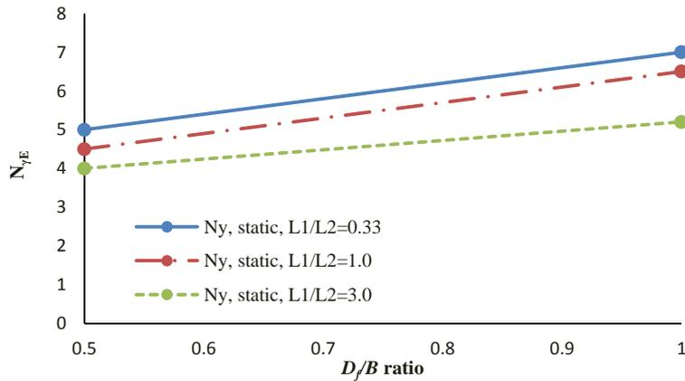
**Fig. 11.** variation of  $N_{\gamma E}$  with  $D_f/B$  ratio with varying layer thickness at static condition
