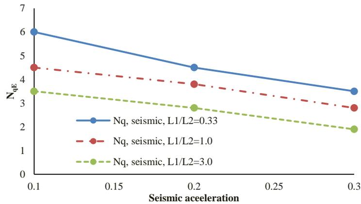
**Fig. 13.** variation of  $N_{qE}$  for  $D_f/B$  ratio=1, with varying layer thickness at seismic acceleration (0.1g to 0.3g)
