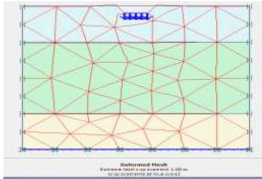
Fig. 3. Deformed mesh of 2m wide strip footing ( $D_f/B = 0.5$ ) for seismic condition for 0.3g
