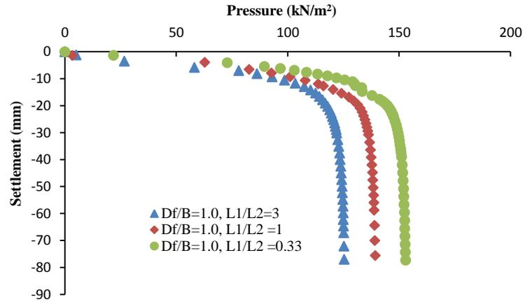
**Fig. 5.** Pressure vs settlement graph for  $D_f/B$  ratio=1 for layer thickness ratio=0.33,1 and 3.0 (seismic case at 0.1g acceleration)
