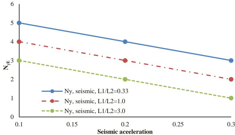
**Fig. 14.** Variation of  $N_{\gamma E}$  for  $D_f/B$  ratio=1, with varying layer thickness at seismic acceleration (0.1g to 0.3g)
