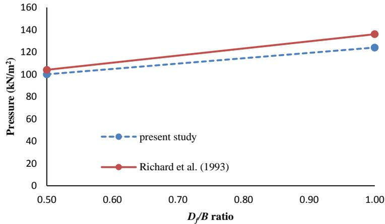
**Fig. 7.** Pressure vs settlement graph for  $D_f/B$  ratio=1 for layer thickness ratio=1 (seismic case at 0.1g acceleration)
