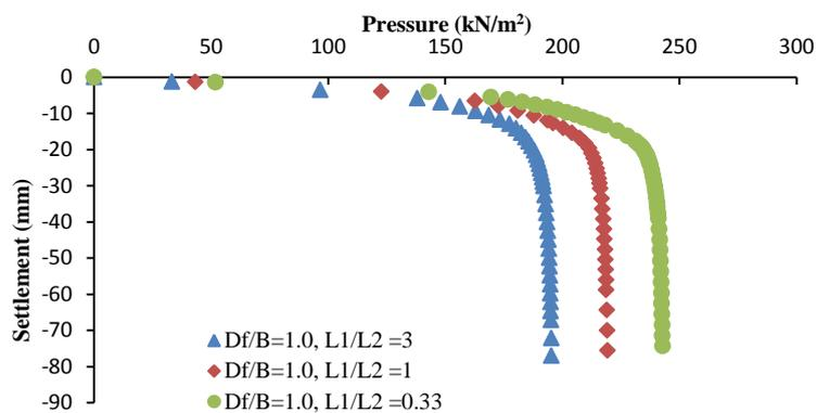
Fig. 4. Pressure vs settlement graph for  $D_f/B$  ratio=1 for layer thickness ratio=0.33,1 and 3.0 (static case)
