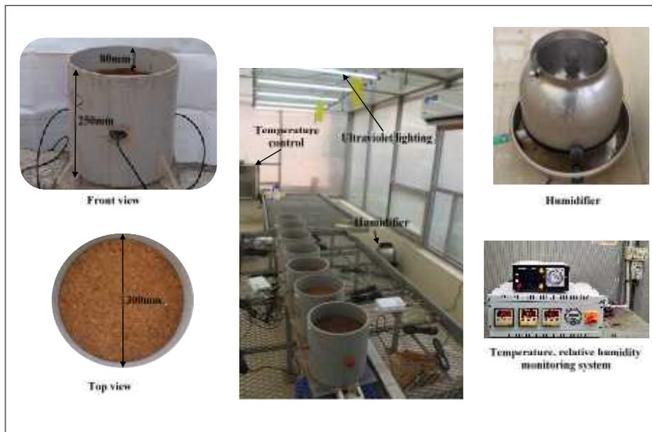
**Fig. 1.** Test set-up for monitoring crack initiation and propagation by image analysis
