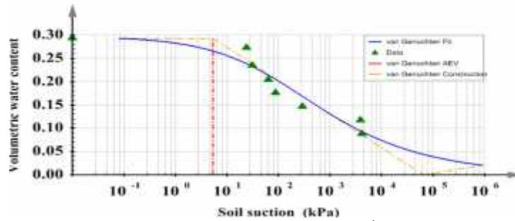
Fig.5.3. Van Genuchten fitting (2<sup>nd</sup> cycle)
