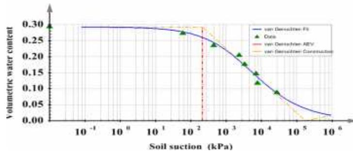
Fig.5.4. Van Genuchten fitting (3<sup>rd</sup> cycle)
