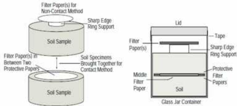
**Fig.2.** Filter paper Method to measure suction
