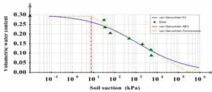
Fig.5.2. Van Genuchten fitting (1<sup>st</sup> cycle)
