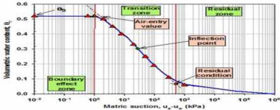
**Fig.1.** Soil Water Characteristic Curve
