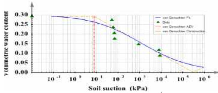
Fig.5.1. Van Genuchten fitting (0<sup>th</sup> cycle)
