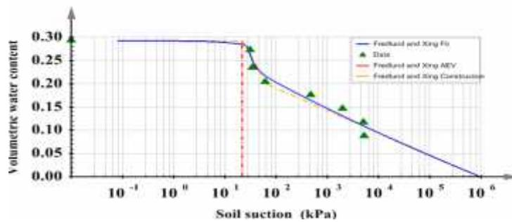
Fig.6.2. Fredlund and Xing fitting (1<sup>st</sup> cycle)
