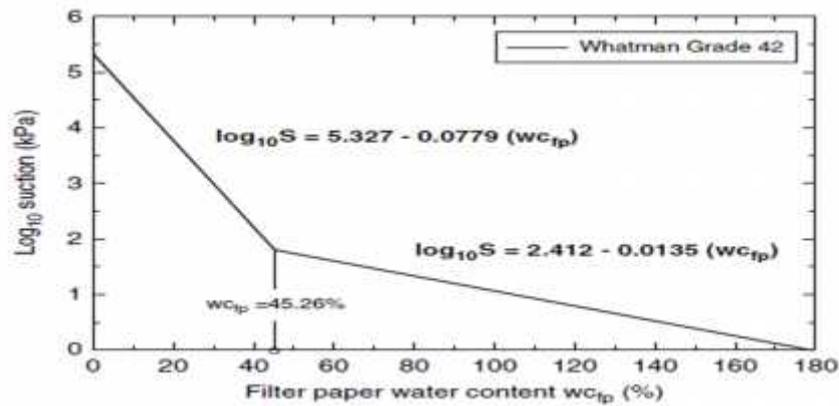
**Fig.3.** Calibration curve for Whatman Grade 42(ASTM D5298-10)
