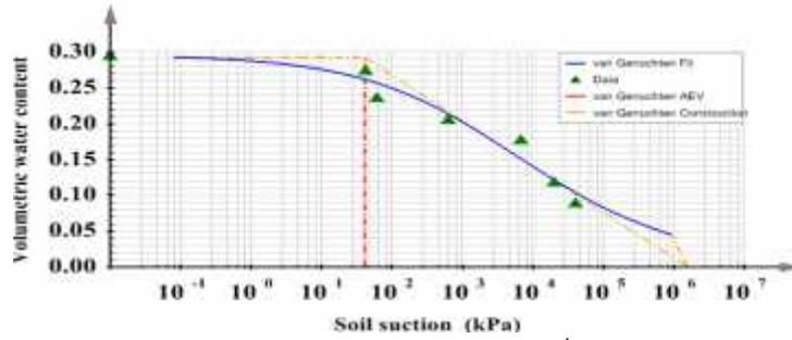
Fig.5.5. Van Genuchten fitting (4<sup>th</sup> cycle)
