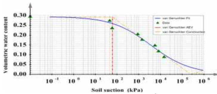
Fig.5.5. Van Genuchten fitting (5<sup>th</sup> cycle)
