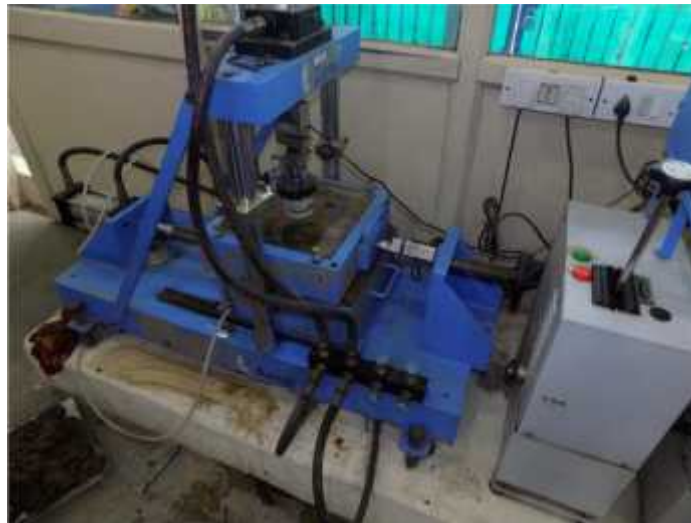
Fig. 1. Large-box Direct Shear Test Apparatus, Aimil make
