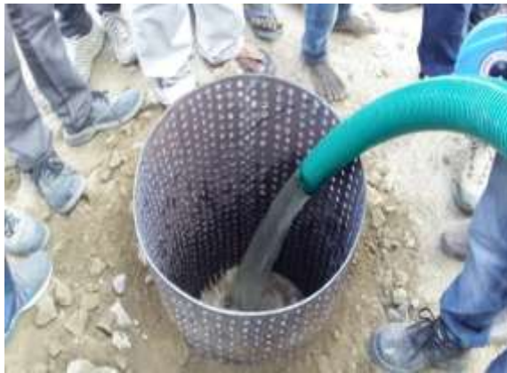
Photo 2: Field Permeability test to determine field permeability of rockfill material
