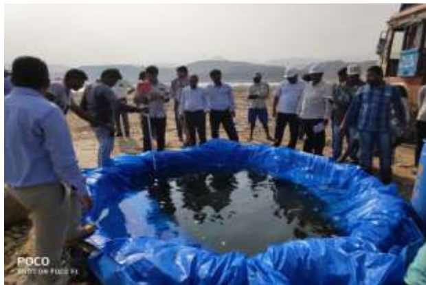
Photo 1: Determination of In-situ density of rockfill material using water replacement method
