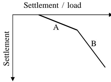
**Fig. 1:** Relationship of settlement and settlement / load
