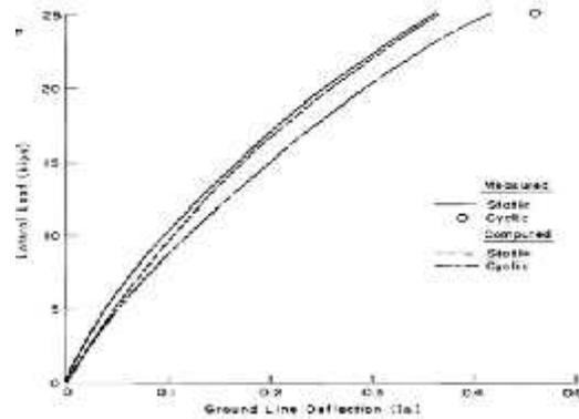
**Fig. 5 :** Comparison of measured and computed deflection for test pile 6 at Arkansas River
