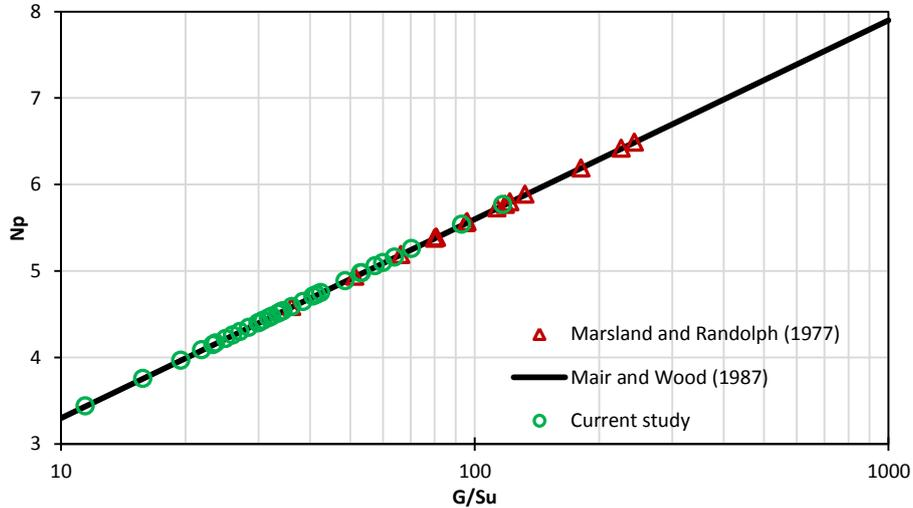
Fig. 4. Variation of pressuremeter constant with shear modulus/undrained shear strength
