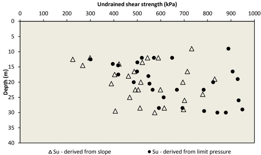
**Fig. 5.** Undrained shear strength derived from pressuremeter test
