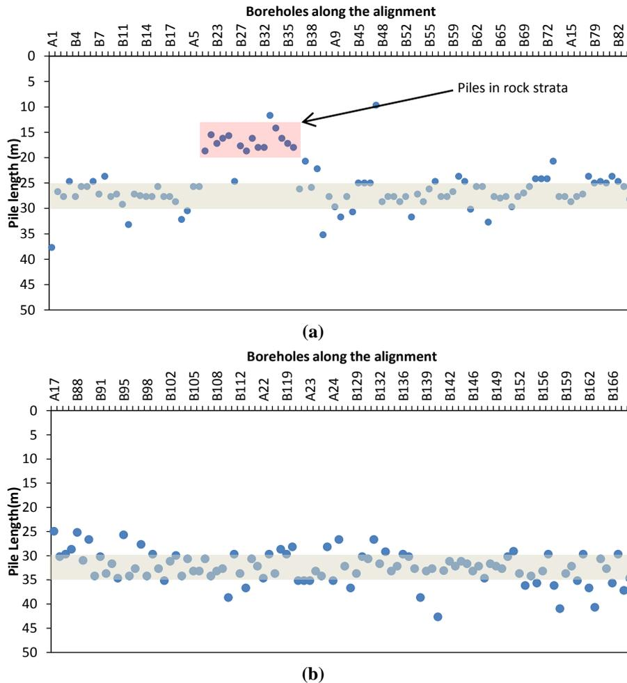
**Fig. 2.** Variation of pile length along the alignment (a) starting from Ch. 0KM to 7.5KM (b) from 7.5KM to 14KM (approx...)
