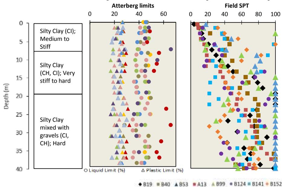
**Fig. 1.** Soil profile and parameters at Pressuremeter locations
