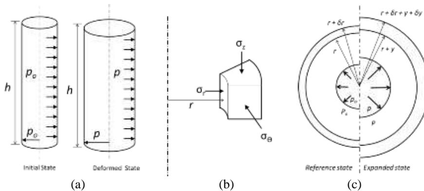
**Fig. 3.** Ideal expansion of cavity (a) expansion of cylindrical cavity (b) Element of soil in cylindrical symmetry (c) reference and expanded stage of cavity at a radius  $r$
