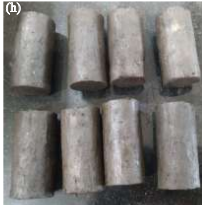
Fig. 3. (a) Extraction of sample from site. (b) Thin tube soil samplers. (c) 3 types of soil samples. (d) Consolidation ring in sampler. (e) Soil sample for consolidation. (f) Extraction of soil sample from sampler for triaxial test. (g) Soil collected in small D samplers. (h) Samples for CU triaxial test.
