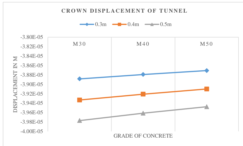
Fig. 5. Displacement of tunnel at crown
