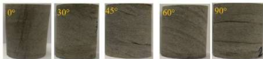
Fig. 2. Prepared specimens for Point load test at different \beta
