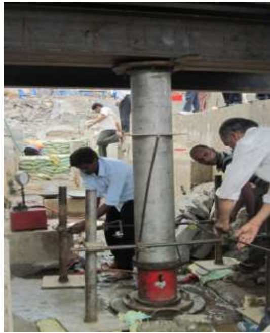
Fig. 6. Setup of plate load test assembly [2]
