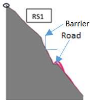
Fig. 6. Slope section RS1 with barrier at an angle of 90^\circ with horizontal.
