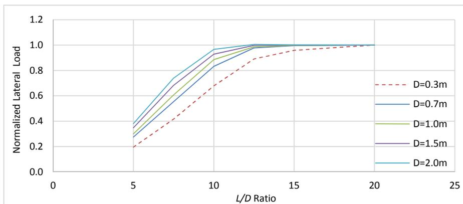
**Fig. 5.** Variation of normalized lateral load with  $L/D$  ratios for different diameters of a pile.
