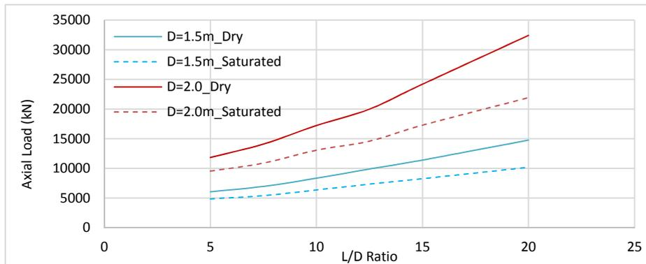
**Fig. 8.** Variation of axial load with  $L/D$  ratios of a pile for different water table conditions.
