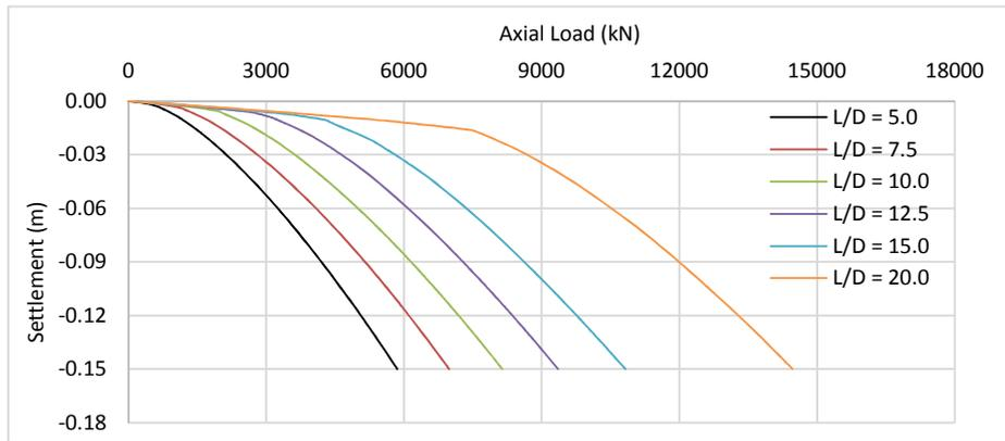
Fig. 4. Variation of axial load with settlement for different  $L/D$  ratios of a pile.
