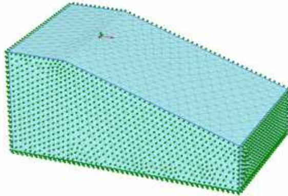
**Fig. 1.** Finite element model of a pile located at the crest of cohesionless soil slope (not to scale).
