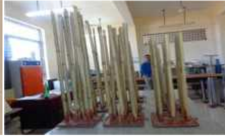
Fig.1. Layouts of single and bamboo pile group. Fig.2 Different slenderness ratios pile groups of bamboo pipe materials model
