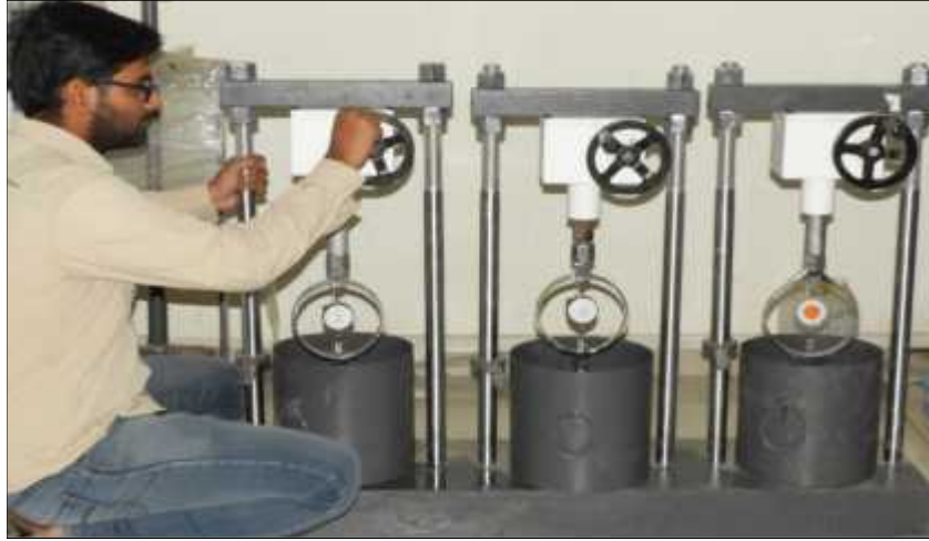
Fig. 2. Swelling test on soil using apparatus
