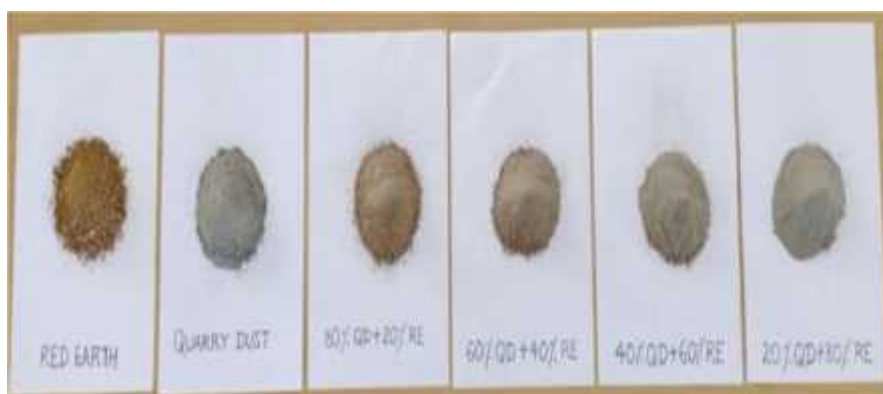
Fig. 1. Quarry dust-Red Earth mixes
