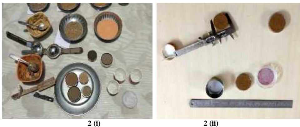
Fig. 2. (i and ii). Dish Method for Determination of Volumetric Shrinkage (%) of Soils.
