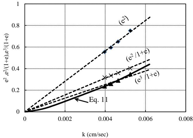
Fig. 4.  $k$  vs. void ratio functions-Ganga Sand
