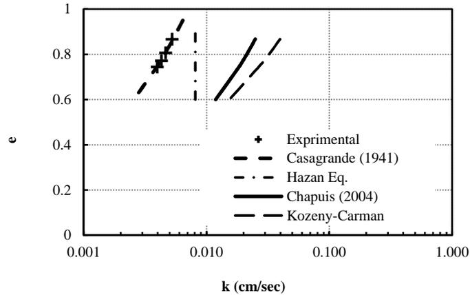
**Fig. 2.** Void ratio vs. coefficient of permeability–Ganga Sand
