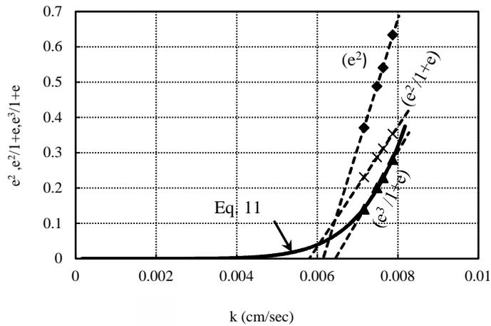
Fig. 5.  $k$  vs. void ratio functions-Ennore Sand
