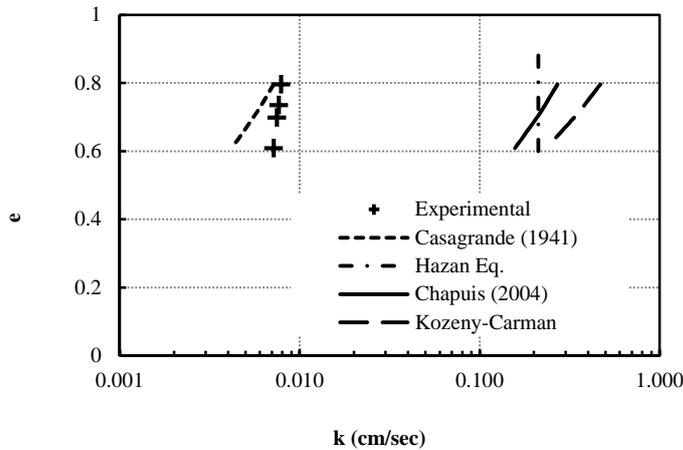
**Fig. 3.** Void ratio vs. coeff. of permeability–Ennore Sand
