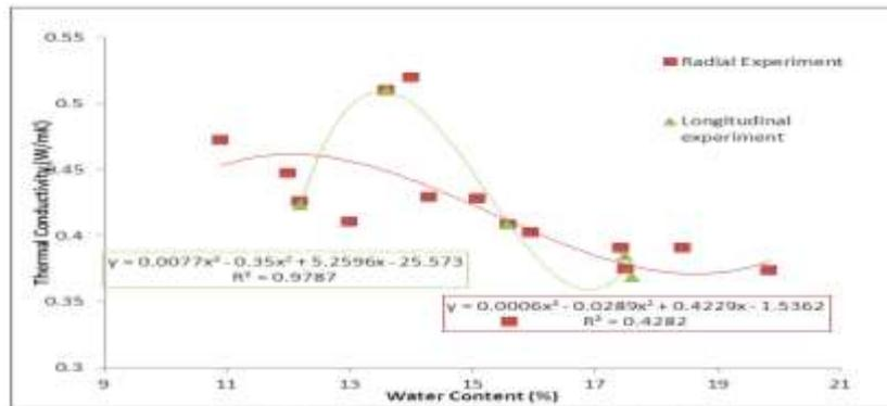
Fig. 16. Water Content v/s Thermal Conductivity
