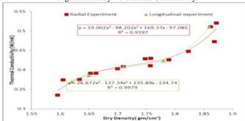
Fig. 18. Dry Density v/s Thermal Conductivity
