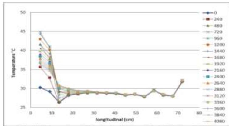
Fig.11 Temperature v/s Longitudinal Distance from Heat Source (Mix 1)
