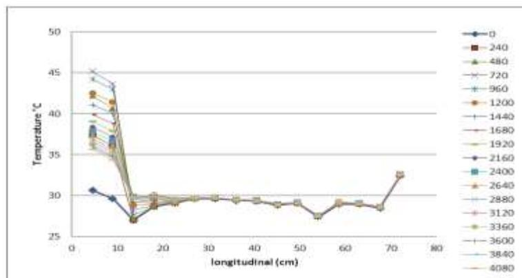
Fig.15 Temperature v/s Longitudinal Distance from Heat Source (Mix 3)
