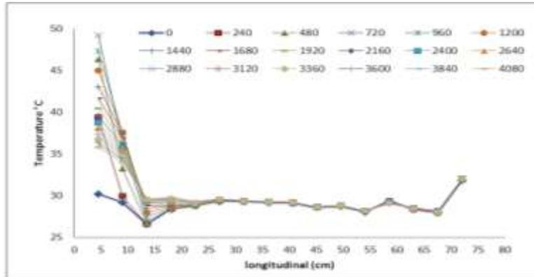
Fig. 13. Temperature v/s Longitudinal Distance from Heat Source (Mix 2)
