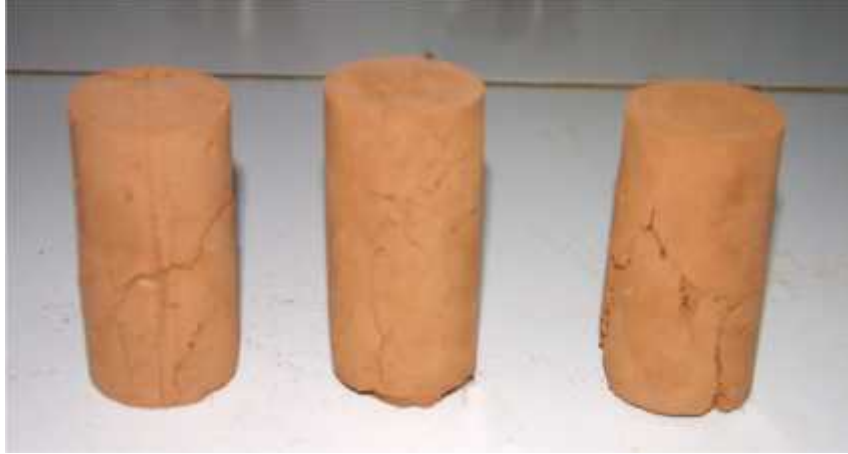
Fig. 1. Failure Pattern Of Cement Stabilized Sample By UCS Test
