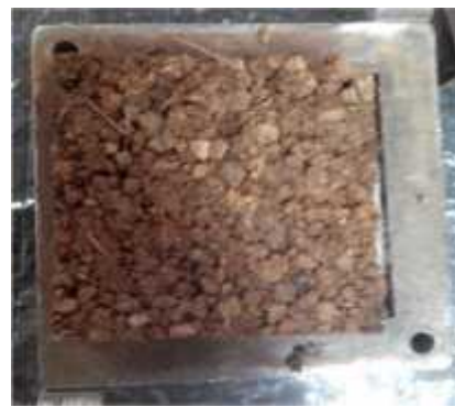
(b) Placement of Powai soil in upper half
