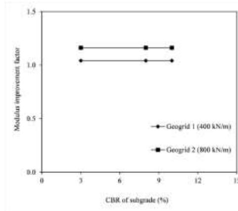
Fig. 2 Comparison of geogrids of different stiffness values based on modulus improvement factor (MIF)
