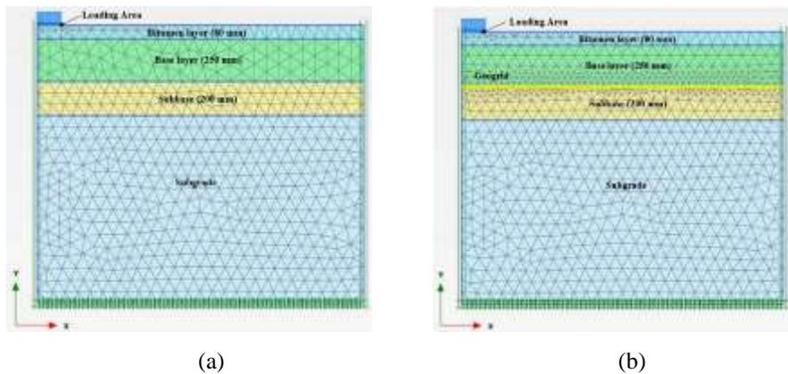
Figure 1. Numerical model for 10% CBR and a 10 msa traffic volume:
