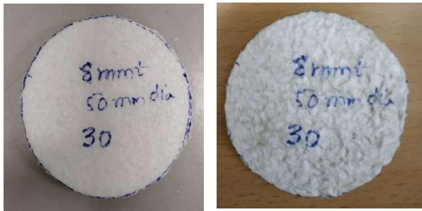
Fig. 9. Geofoam sample before and after the test
