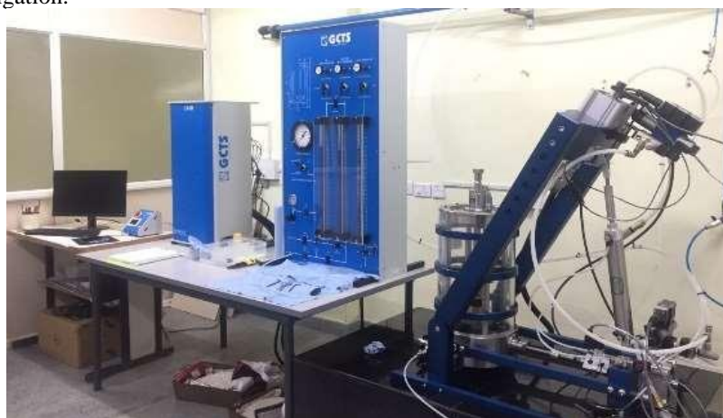
Fig. 4. Cyclic simple shear test setup at IISc Bangalore
