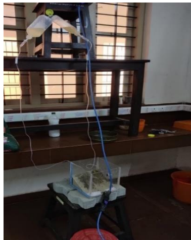
Fig. 6. Gravity Flow method for MICP treatment
