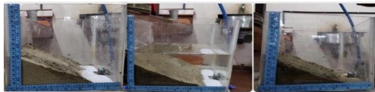
Fig. 10. Slope S80M20 failure during simulated tidal cycle (untreated)
