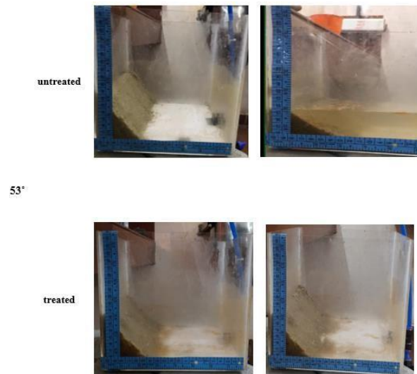
Fig. 7. Slope failure and erosion (35° untreated and MICP-treated slope after tidal events.)
