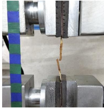
Fig. 2 Tensile testing set-up in UTM
