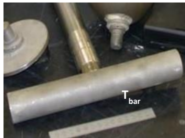
Fig.1. Photograph of a T bar (Yafrate et al. 2007)
