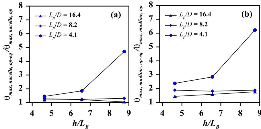
Fig. 5. Variation of ratio of rotation due to operational and seismic load and operational load at (a) tower top and (b) monopile at mudline in the side-side direction.
