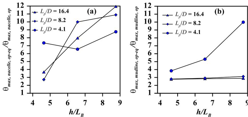
**Fig. 6.** Variation of ratio of rotation due to operational and seismic load and operational load at (a) tower top and (b) monopile at mudline in the fore-aft direction.
