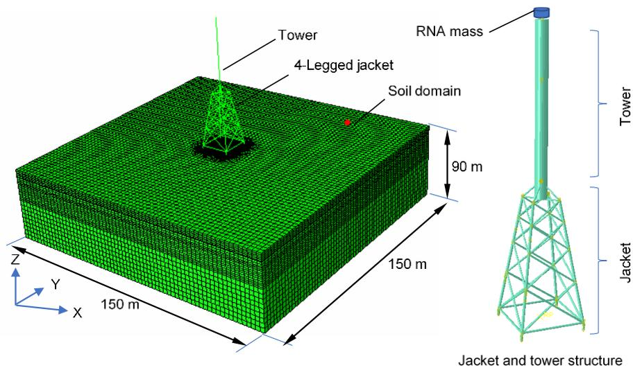
**Fig. 1.** 3D numerical model of jacket supporting 10 MW wind turbine.
