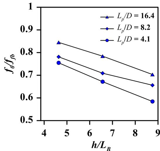
**Fig. 3.** Variation of the natural frequency with respect to aspect ratios of pile and jacket.
