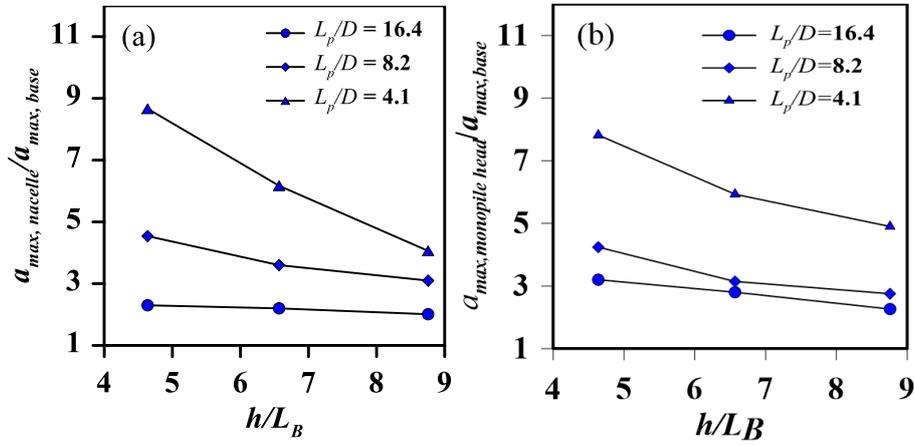
Fig. 4. Amplification of maximum vertical acceleration: (a) at the tower top and (b) monopile head.
