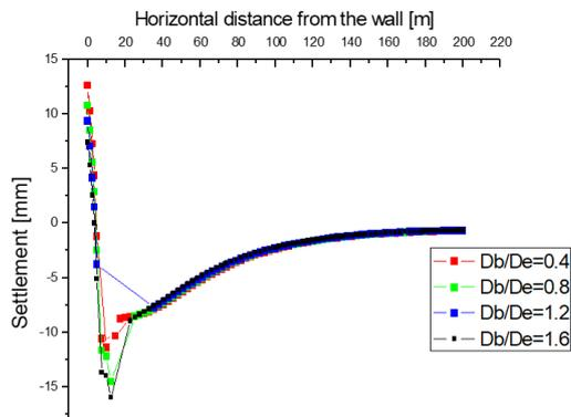
Fig. 7. Variation of vertical settlement with horizontal distance from the wall for  $D_e=10m$ .
