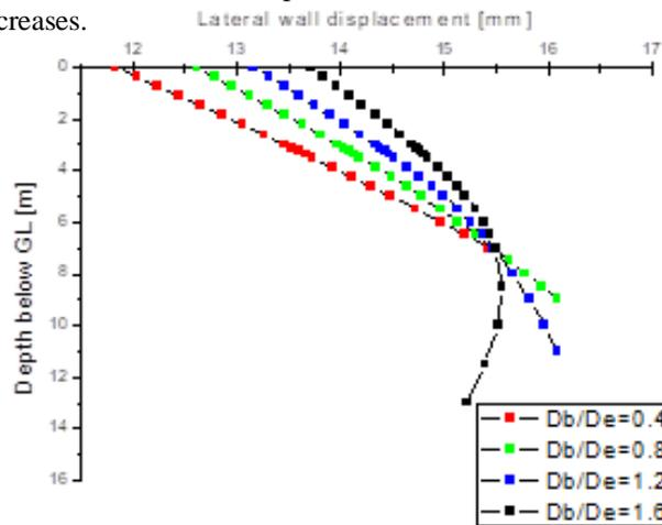
**Fig. 3.** variation of Lateral wall displacement with Depth below GL for  $D_e=5\text{m}$
