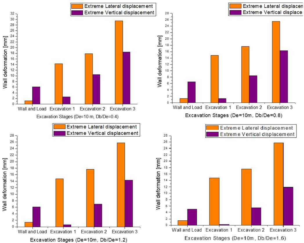
Fig. 10. Behaviour of Wall at different Excavation Stages ( $D_e = 10m, D_b/D_e = 0.4, 0.8, 1.2, 1.6$ )
