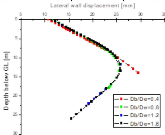
**Fig. 4.** variation of Lateral wall displacement with Depth below GL for  $D_e=10\text{m}$
