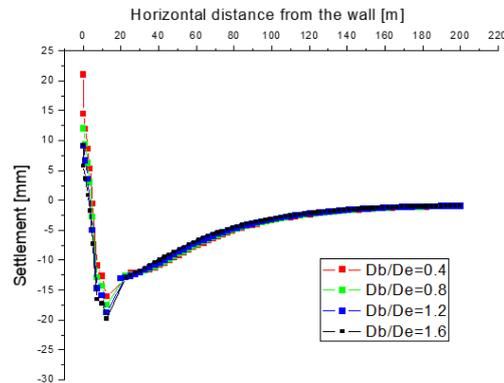
**Fig. 8.** Variation of vertical settlement with horizontal distance from the wall for  $D_e=15\text{m}$ .
