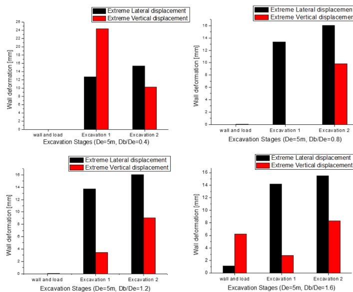
**Fig. 9.** The behavior of Wall at different Excavation Stages ( $D_e = 5\text{m}$ ,  $D_b/D_e=0.4, 0.8, 1.2,$  and  $1.6$ )
