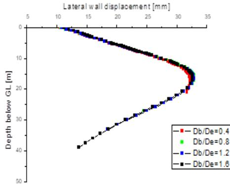
Fig. 5. variation of Lateral wall displacement with Depth below GL for  $D_e=15m$ .
