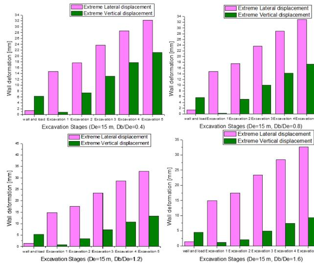
**Fig. 11.** Behaviour of Wall at different Excavation Stages ( $D_e=15\text{m}$ ,  $D_b/D_e=0.4, 0.8, 1.2, 1.6$ )
