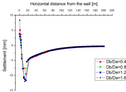
Fig. 6. Variation of vertical settlement with horizontal distance from the wall for  $D_e=5m$ .
