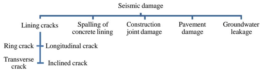
**Fig. 3.** Different types of seismic damage in tunnel
