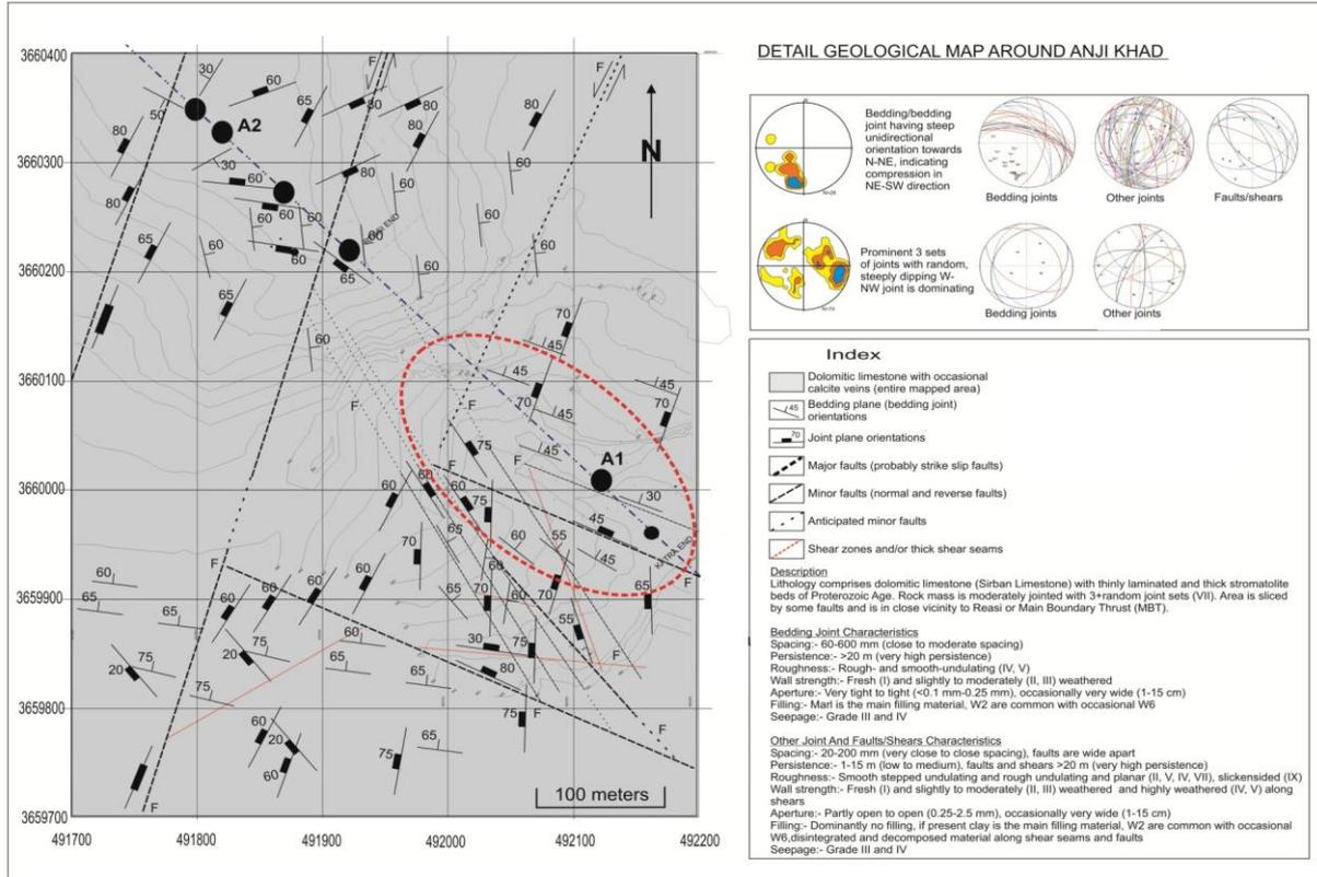
**Fig. 2.** Detail Geological map around Anji Khad , Reasi, Jammu & Kashmir, India. A1 and A2 are the locations of in-situ shear tests of Singh and Sarwade (2015)
