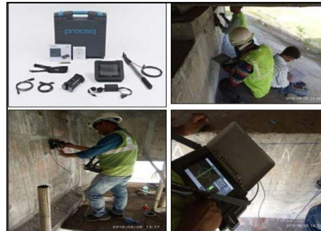
Fig. 6. Profometer Scan Test
