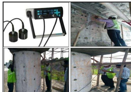
Fig. 4. Ultrasonic Pulse Velocity Test
