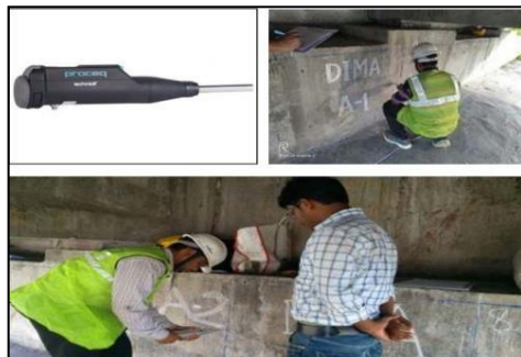
Fig. 3. Rebound Hammer Test
