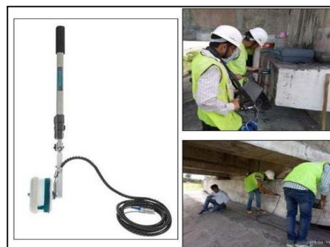
Fig. 7. Half Cell Potential Test
