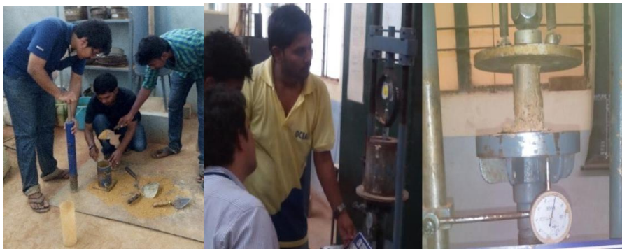
Fig. 2. Sequence of Compaction, CBR and UCS Testing of Soil Samples.
