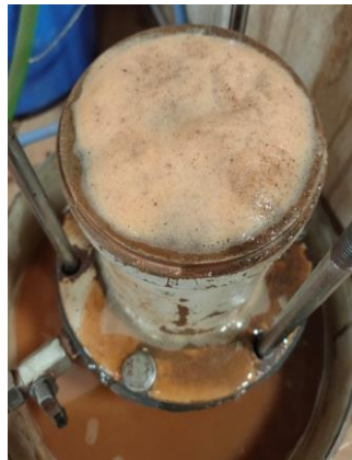
Fig. 6. Piping failure in river sand
