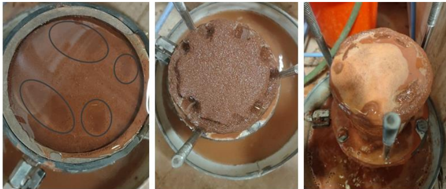
Fig. 4. Piping failure observed in red soil
