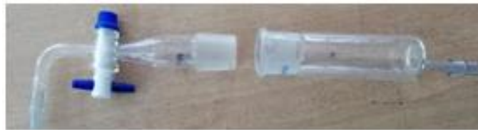
Fig. 1. The glass tube of pinhole apparatus.
