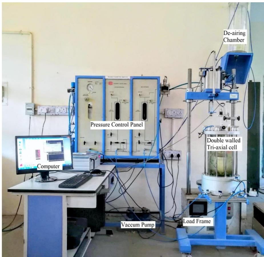
**Fig. 4.** Dynamic Triaxial testing apparatus used in the present study.
