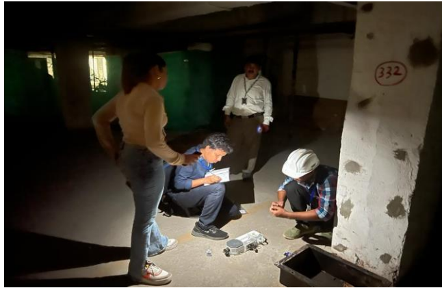
Fig.12. Placing geophones for vibration measurement in Aster-2
