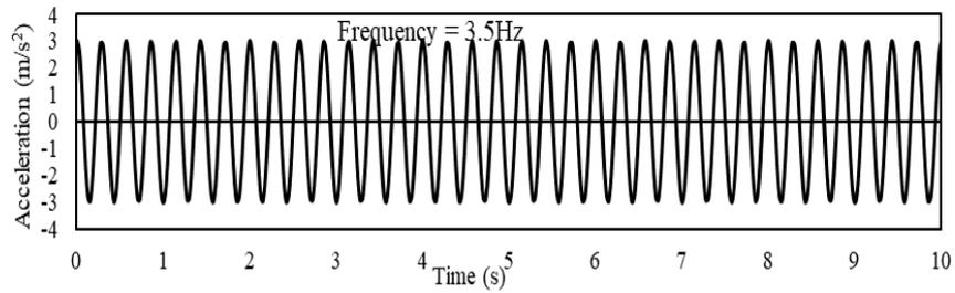
Fig. 2. Harmonic Excitation time histories of frequency,  $f = 3.5\text{Hz}$  with amplitude  $3\text{m/s}^2$
