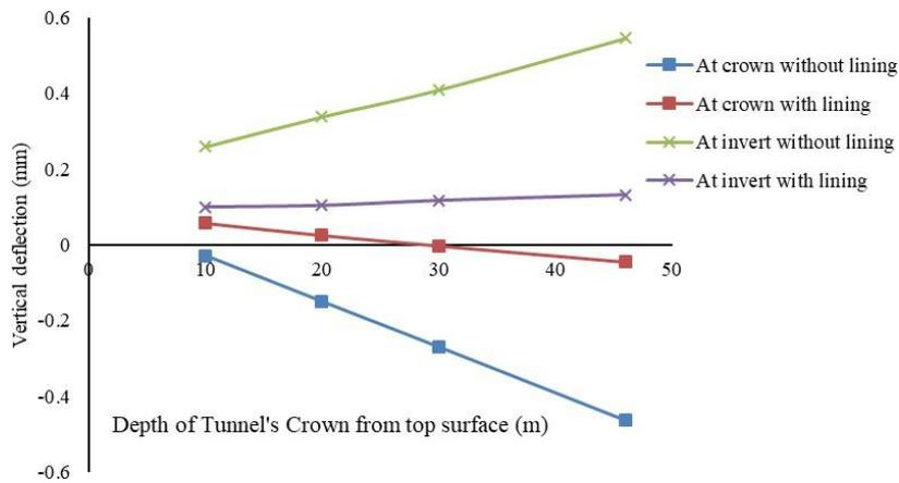
**Fig.4.** Comparison of vertical deflections at the crown and invert under static conditions
