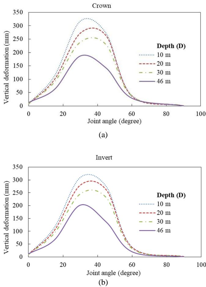
Fig. 8. Comparison of vertical deformation at tunnel (a) crown and (b) invert due to harmonic excitation of 3.5Hz frequency
