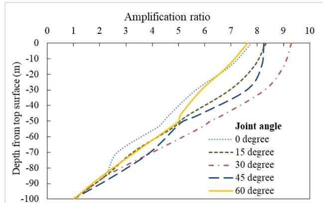
**Fig. 5.** Amplification of amplitude in the rock mass for different joint angles at frequency  $f = 3.5\text{Hz}$
