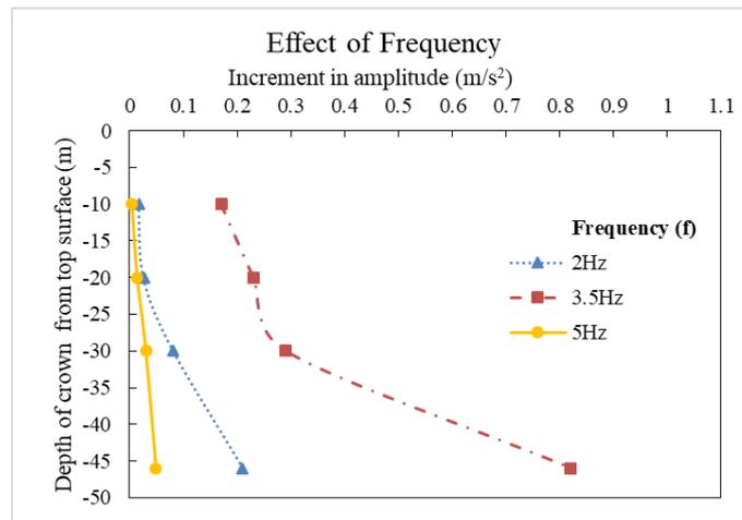
**Fig. 7.** Increment in the response due to presence of tunnel for joint angle  $30^0$
