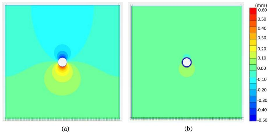
Fig. 3. Deformations in the rock mass when tunnel is at the center i.e. at depth 46m (a) without lining and (b) with lining
