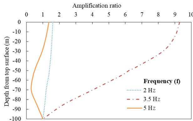
**Fig. 6.** Effect of frequency of excitation on amplification without tunnel for joint angle  $30^\circ$
