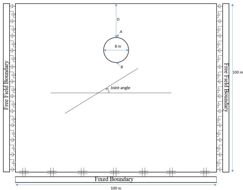
**Fig. 1.** Geometry of rock mass and tunnel with boundaries
