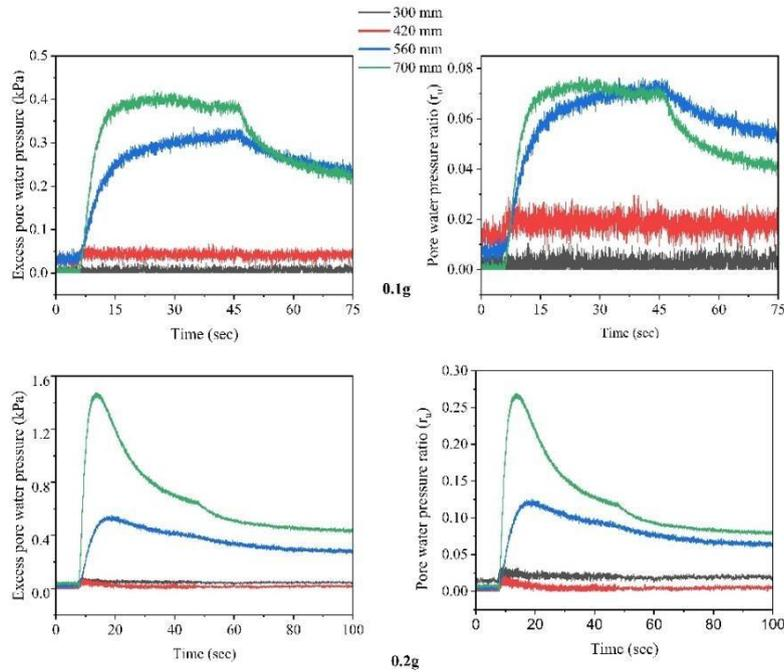
**Fig.6.** Developed excess pore water pressure and pore pressure ratio during 0.1g and 0.2g input motion
