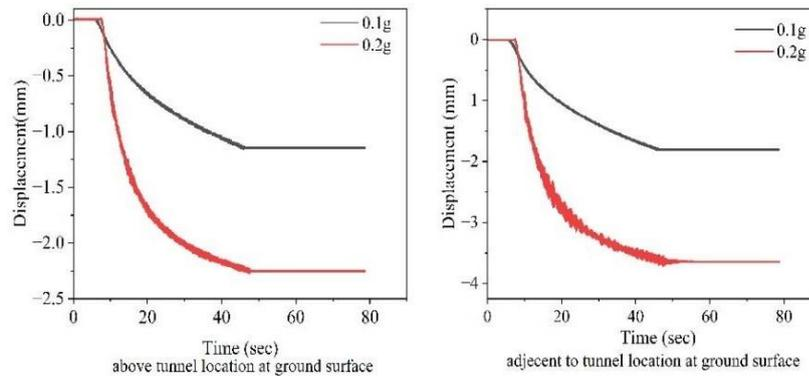
**Fig.5.** Displacement of soil during 0.1g and 0.2g input motion
