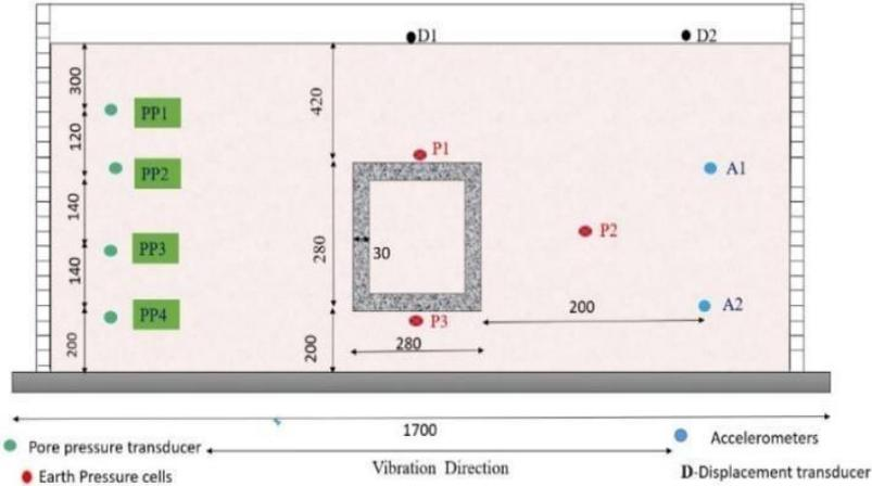
Fig.2.Sensor arrangement for experimental test program
