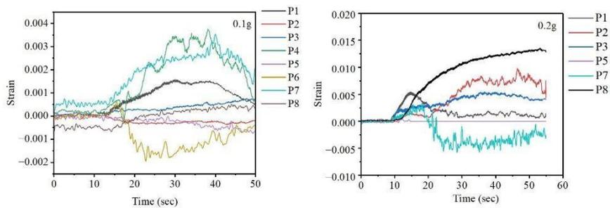
**Fig.8.** Strain developed at different locations of the tunnel
