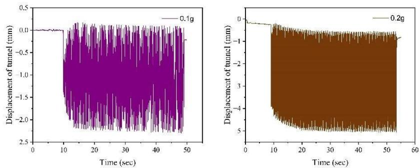
**Fig.7.** Displacement of tunnel obtained from DIC during 0.1g and 0.2g input motion
