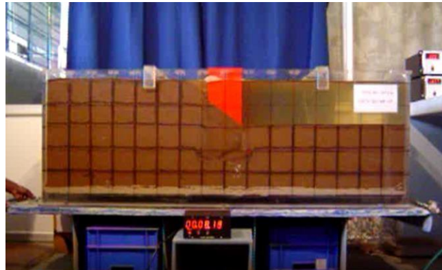
Fig.17: Assembly of quay wall model in manual shaking table with transparent model container (Nanjundaswamy P. (2008))
