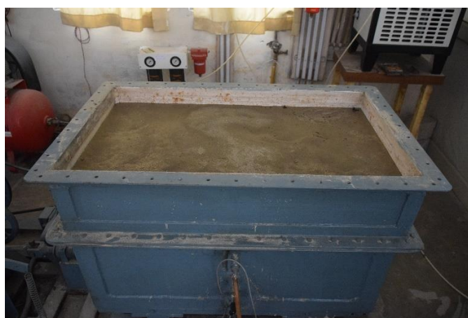
Fig. 2. Prepared sand specimen at desired relative density
