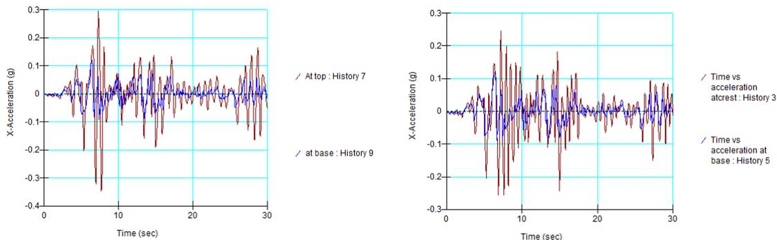
Fig 4: Time versus Acceleration graphs at crest and base without and with dense wall
