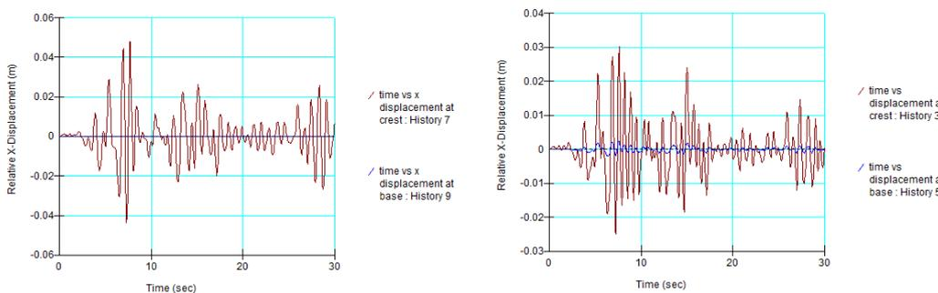
Fig 5: Time versus Horizontal Displacement graphs at crest and base without and with dense wall
