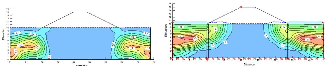
Fig 6: Excess pore water pressure for the dam without dense wall and with dense wall
