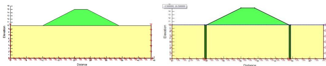
Fig 1: Earthen dam without Dense wall and with dense wall provided in the foundation soil
