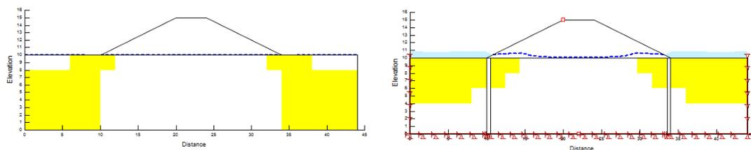
Fig 7: Liquefaction zone for the dam without dense wall and with dense wall
