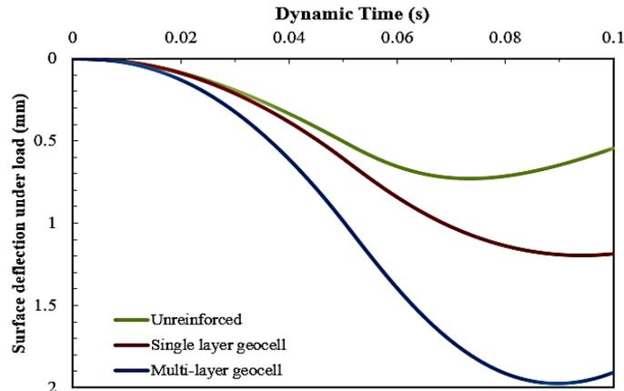
Fig. 5. Dynamic time vs. surface deflection under the wheel load
