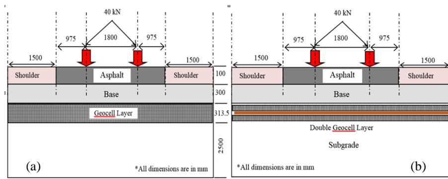
**Fig. 2.** Pavement structure with (a) single and (b) double layer geocell reinforcement
