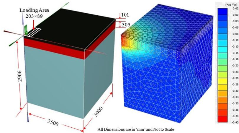
Fig. 3. Validation of Saad et al. [12] using Plaxis3D
