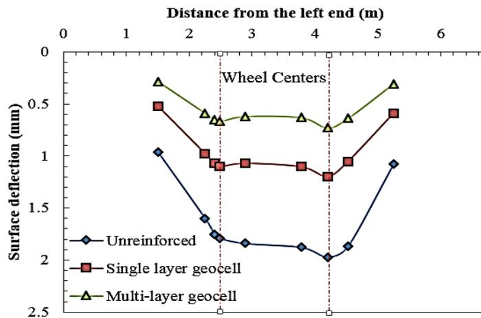
Fig. 6. Deflection at different locations of the pavement sections
