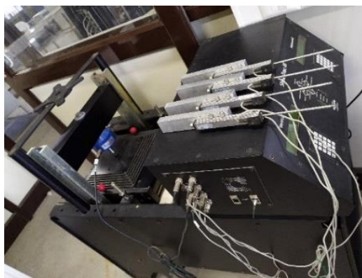
Fig. 4. Large direct shear testing equipment
