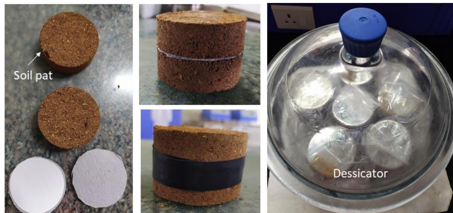
Fig. 5. Filter paper method for the determination of SWCC of the soil
