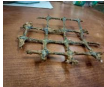
Fig. 4. Exhausted geogrid after the test
