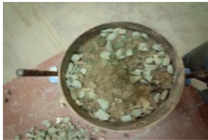
Fig. 3. Intermixing of soil and aggregate layer in the unreinforced system
